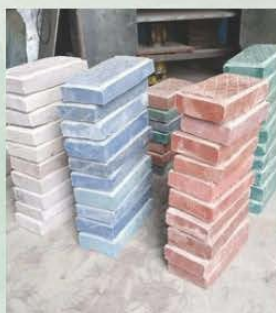
Recycled bricks produced by Gjenge Makers Ltd.
